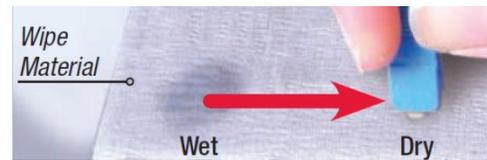
Figure 7 – Combination Cleaning process
